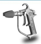
This lightweight drop-forged, manual spray gun, (for applying various maintenance and decorative finishes) features a stainless steel head and fluid passages, ball-type fluid valve, removable valve assembly, tungsten carbide seat, and built-in diffuser. The thumb-operated safety trigger lock permits one hand locking, unlocking, and triggering. A tip guard is included for added safety. (*Maximum operating pressure is 6000 PSI.*) Part Sheet: 77-2340. (*Spray tip not included. order separately*)
